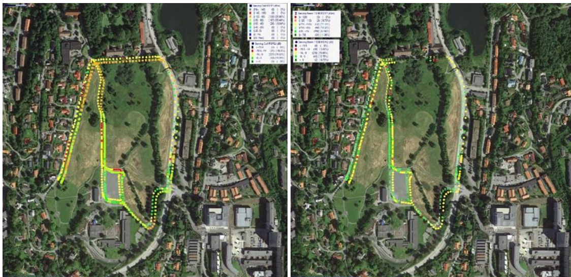
Figure 87. 2.3GHz (left) and 3.6 GHz (right) coverage map. RSRP and RSRQ values.
