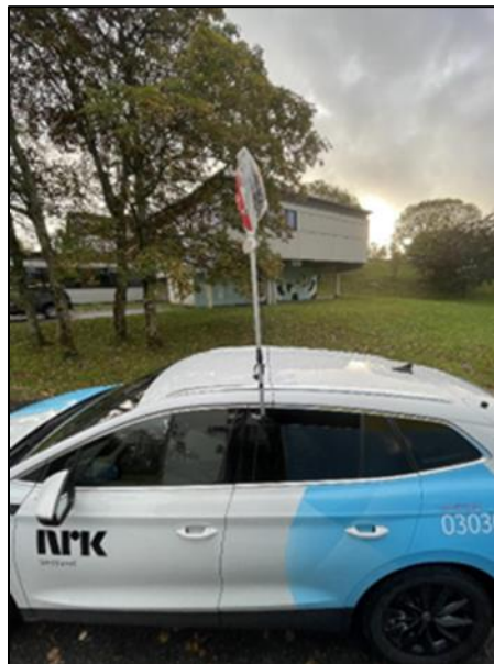
Figure 92. Car with a 5G phone on a mast.
