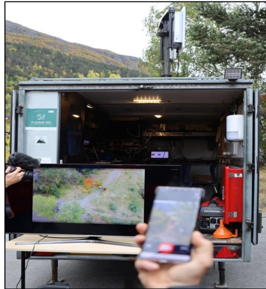
Figure 20. Nemergent PTT application group call transmission and drone video on a screen.
