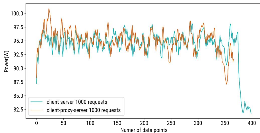
Figure 79. Power dissipation of client-server and client-proxy-server setup with 1000 requests.
