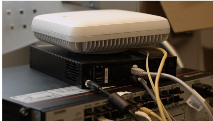
Figure 17. O2M CBCF on CumuCore 5GC with Huawei gNodeB on top.
