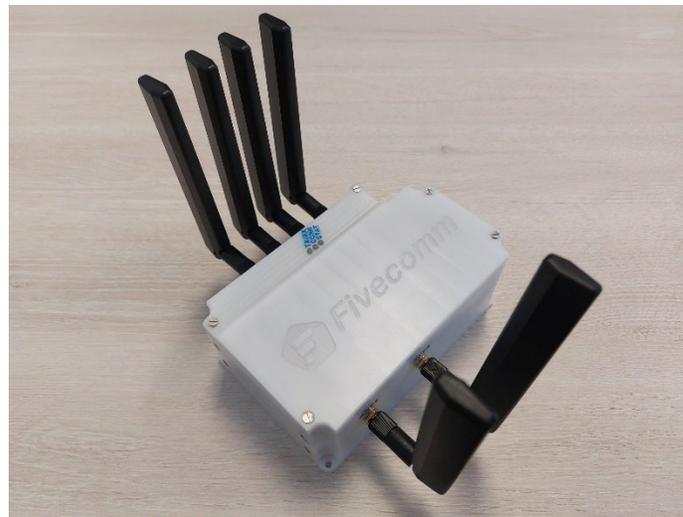
*Figure 15: 5G modem developed by Fivecomm and validated in ABB lab, as part of UC4 final trials.*
