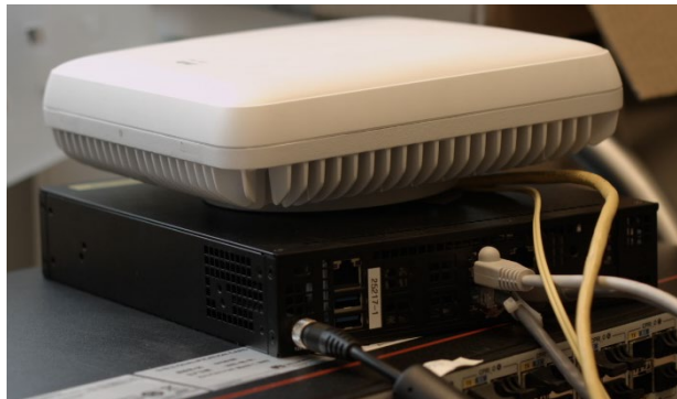
Figure 34: One2Many-Everbridge CBCF on-boarded in Cumucore 5GC box connected to a Huawei LampStation (White box)
