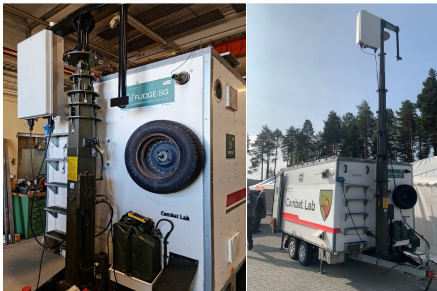
Figure 13: Huawei AAU mounted on the NOW mast in retracted and deployed position.
