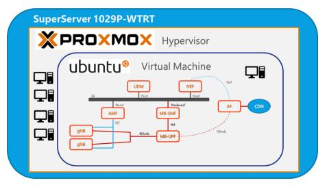
*Figure 20: Deployment architecture of the UPV node, showcasing the 5MBS prototype.*
