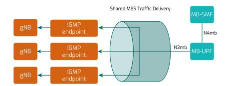
Figure 19: Open5GCore Release 6 5MBS implementation by UPV. An IGMP endpoint is deployed for every virtual gNB instanced for the experiment, which will translate the multicast IP from a multicast flow into a unicast one.
