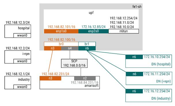
Figure 18: IP Routing Configuration of User Plane
