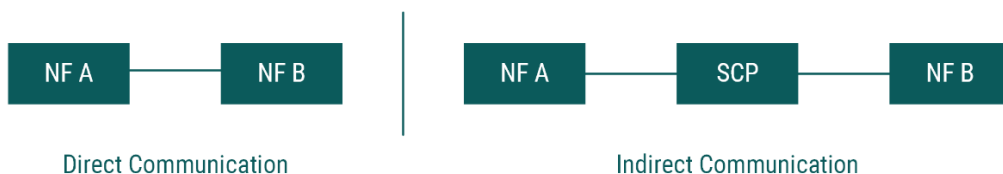
Figure 3-1: Direct and indirect communication options based on Release 16 [3GP19b]
