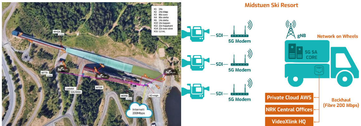
Figure 6: Midstuen deployment topology (right) and the map of the location (left), including the position of the NoW and the cameras
