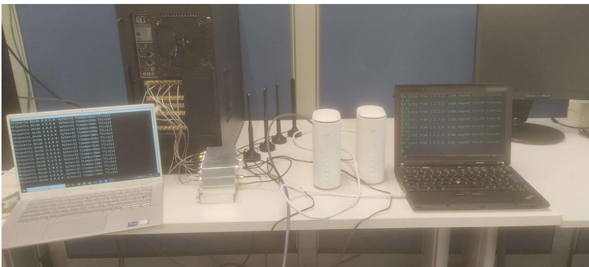
Figure 37: Integration of 5G core with Amarisoft RAN at UPV
