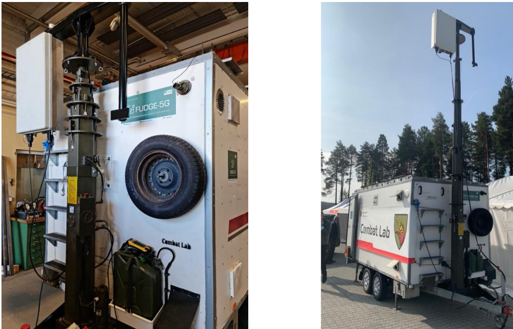
Figure 2: Network on Wheels (NoW) with the mast retracted (left) and deployed (right). Huawei 5GRAN is mounted on the mast.
